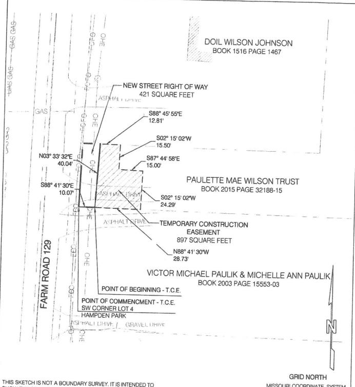
THIS SKETCH IS NOT A BOUNDARY SURVEY. IT IS INTENDED TO SHOW THE CONFIGURATION OF A TEMPORARY CONSTRUCTION EASEMENT.
